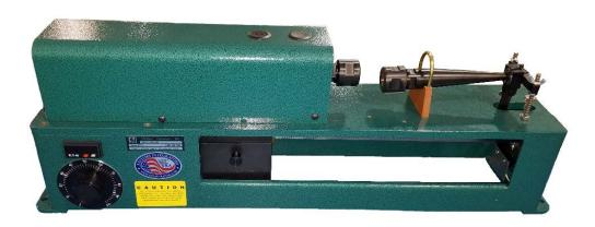
Systems Integrators and our RBF model line of rotating beam fatigue machines accurately and economically test a broad range of materials and under reverse bending stress. Accurate test results require high quality, consistent test specimens. Fatigue Dynamics has helped numerous customers in this critical phase of fatigue testing and has produces tens of thousands of test specimens. You can prepare your own test specimen or have Fatigue Dynamics prepare them for you!
